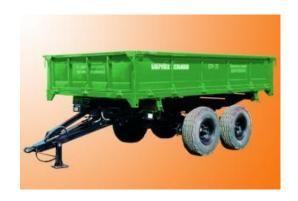
Building-block design, tractor of class 1,4-2,0. Semitrailer without patched on boards PTU-7,5 is intended for transportation of various building dry loads and agricultural dry loads: root crops, organic fertilizer with unloading from 3 sides.
